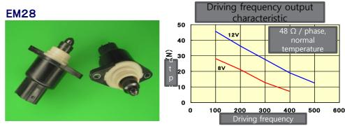
· Output characteristics are DC12V, continuous energization · specification · Specified for linear drive, flow control, valve drive is possible
